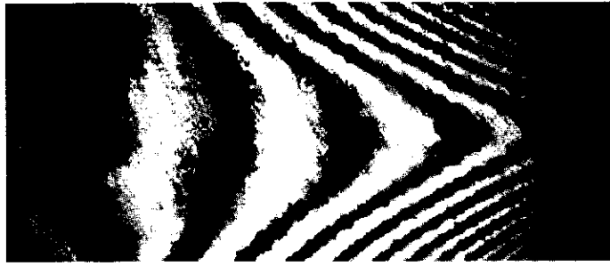
Fig. 1a. Measured double-pass Fizeau interferogram at 532-nm wavelength.
