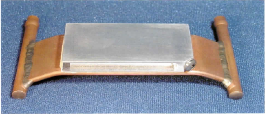
Fig. 15. PCC composite TES mounted to Lytron cold plate.
