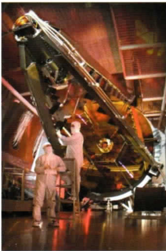
Fig. 3. Left: ALI beam director (Griff Telescope) employing the 4-m LAMP mirror. Right: U.S. Air Force Academy design for reusing the LAMP mirror in an astronomical and space surveillance telescope.
