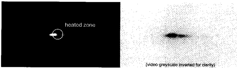
Fig. 10. Frame from high-speed video showing double-site crack initiation for 0.025-in. (0.635-mm)-thick dogbone specimen at 90% yield subjected to 0.40-in. (1-cm)-diameter IR heating at 1 \text{ kW/in.}^2 ( 155 \text{ W/cm}^2 ).
