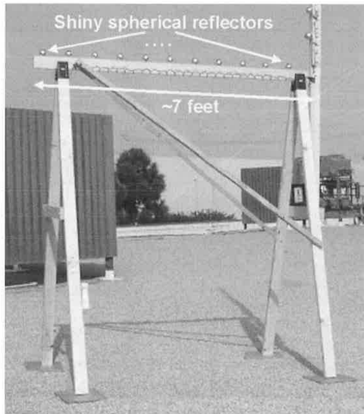
Fig. 2. Spherical reflectors on wooden sawhorse on O2 roof. (The vertical spar that is partially shown in the photograph was removed prior to the experiment. Golden colored spheres were replaced with silver colored ones prior to the experiment.)
