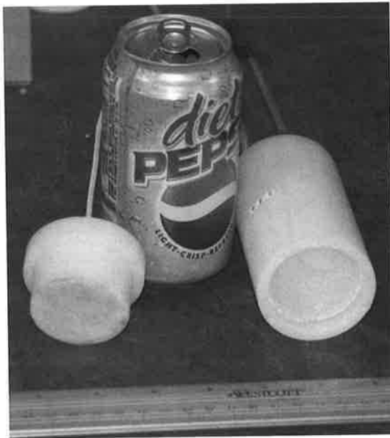
Fig. 6. Typical miniature Loki explosive-driven, 140-kV FEG.
