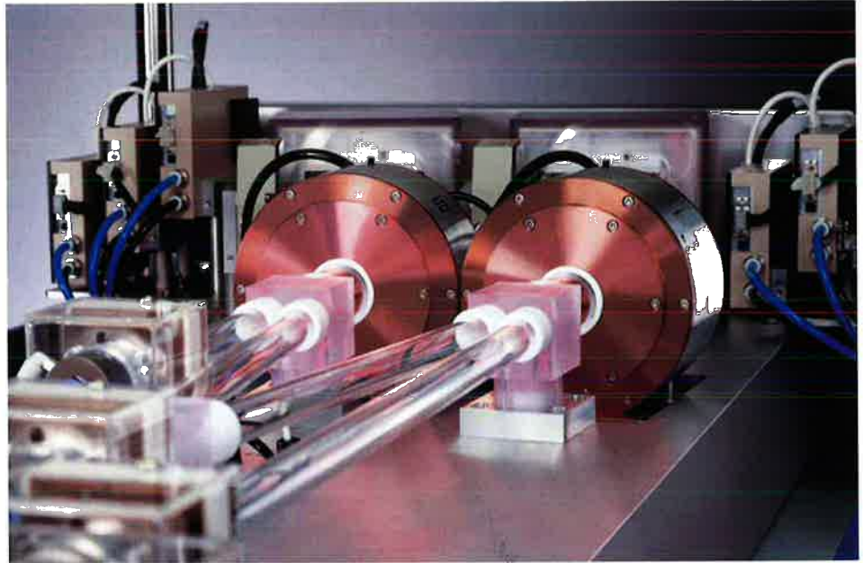
Fig. 21. One-kilowatt, thin disk laser for materials processing (courtesy of Trumpf-Laser).
