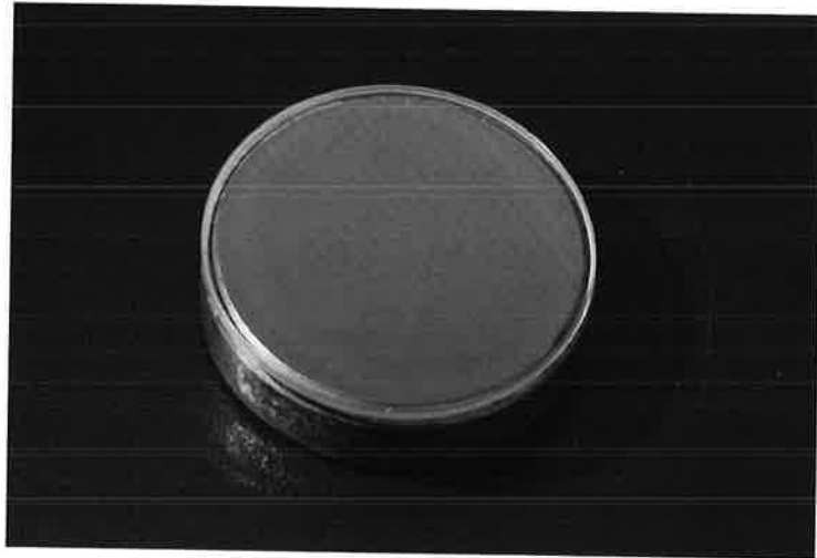
Fig. 19. CADB-bonded YAG-CuW structure (Sample C) with HR coating at the interface.
